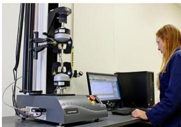
With the increasing industry demand, Savant Labs has recently added the capability to perform seal, (also called elastomer), compatibility testing. Seal compatibility testing is an important element of oil specifications to ensure that oil formulations are compatible with the gasket and sealing materials used in modern vehicles.
