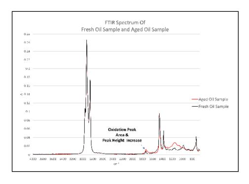
The degree of oxidation is measured by FTIR in accordance with ASTM D7214 which quantifies the Peak Area Increase (PAI) in the carbonyl region.
