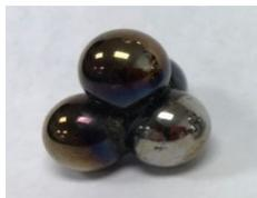
When the extreme pressure test fails, this is called welding. There are certain attributes to look for. They are: a sharp transverse movement of the friction force, an increased noise level of motor, smoking from test-oil cup, a sudden drop in the lever arm, or the motor comes to a complete stop, indicating the balls have welded.
