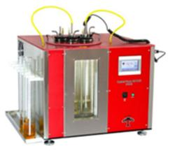
pumping, and splash lubrication. These tests measure both the volume of foam formation and the stability (amount of foam left as a function of settling time).
