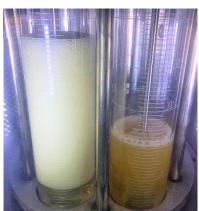
the oil up to the surface. The right cylinder in this image demonstrates kinetic foam where there is air dispersed
