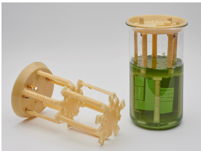
Figure 3. (Left) The wire and test fluid positioned for the WCT test. (Right) The WCT underway. Photos provided courtesy of Lubrizol Corporation and used with permission.
